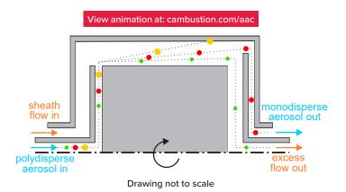
With the classifier stationary, all particles follow the sheath flow, and are lost in an internal HEPA filter.
